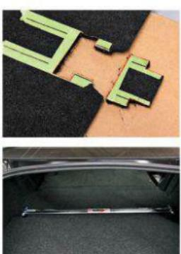
With the rear bar came instructions on exactly how much to cut the rear carpet for a perfect fit.
