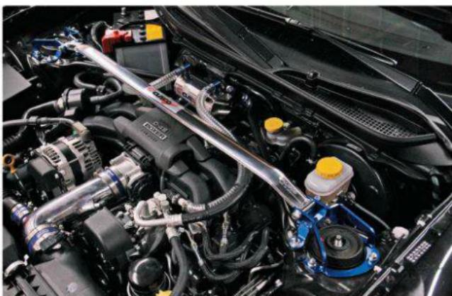
Wanting a bit more chassis tuning, we ordered the Cusco Type OS strut tower bars. The great thing about the Cusco unit is the optional BCS (brake cylinder stopper) that is incorporated into the end bracket. These bars will go on top of the KW coilovers to keep the suspension geometry and chassis from flexing too much.
