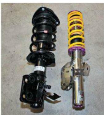
KW versus OEM suspension.
