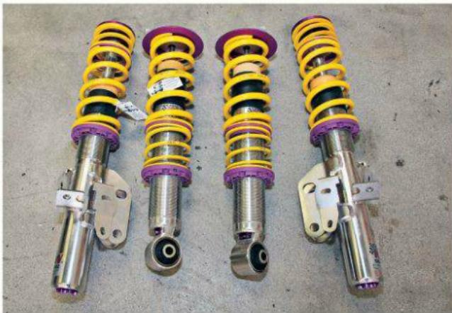
KW Variant 3 coilovers with 14-level adjustable compression damping.
