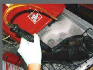
The environmentally friendly, water-soluble solution flows through a cleaning brush, making cleanups a snap and a sealable lid keeps the tank clean and neat when not in use.
